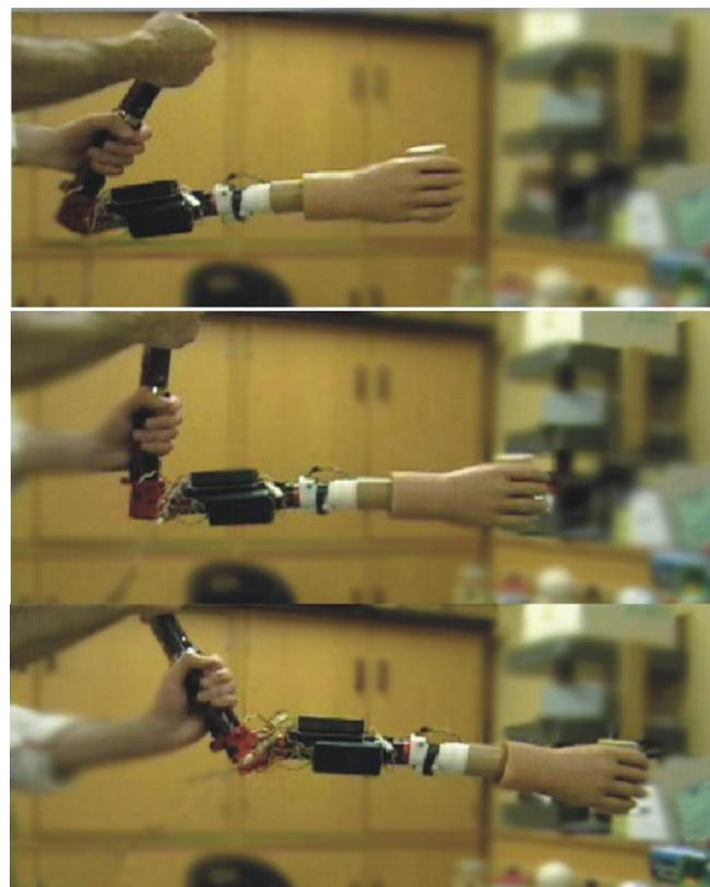
Fig. 9. **Motion Compensation** - The humeral section flexes and extends and the motion is detected by the accelerometers in the wrist and the elbow is driven to compensate for the motion.
