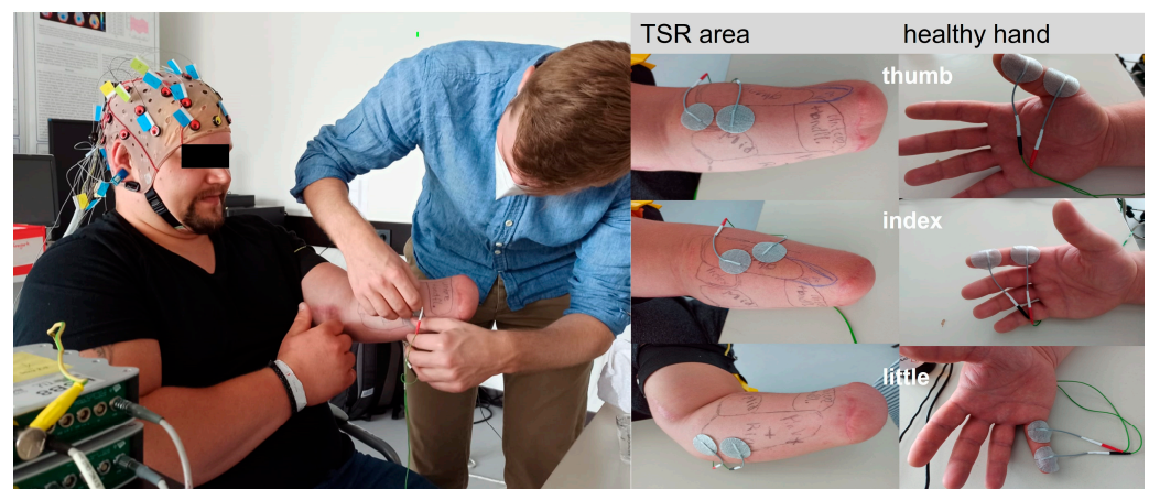
Figure 3. Experimental setup for SEP measurement. (Left) EEG cap attached and setup of electrodes at stimulation areas. (Middle) Electrode placement for stimulation of thumb, index, and little finger. (Right) Stimulation setup for thumb, index, and little finger on the healthy hand.
